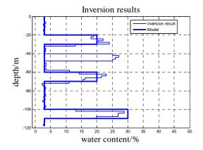
Figure 3. The Inversion Results for Three Layers without Noise
