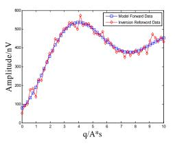
Figure 6. The SNMR Forward of 3-layer Aquifers and the Reforward of RSATA with Noise of s/n=20dB Inversion Results
