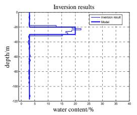
Figure 2. The Inversion Results for Single Layer with Noise of s/n=20dB
