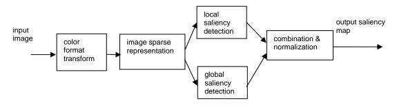
Figure 2. The framework of our proposed model
