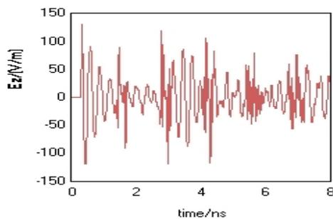
Figure 5. Electric Field of the Place 3cm to the Square Annular Aperture in the Cavity
