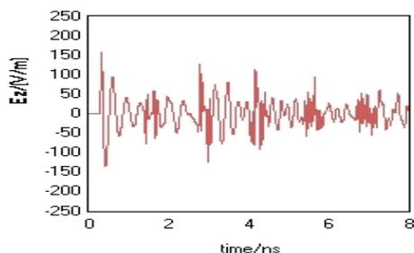
Figure 9. Electric Field of the Place 3cm to the Aperture in the Cavity when  $L=30\text{MM}$ ,  $W=16\text{mm}$
