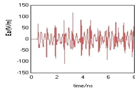
Figure 6. Electric Field of the Center of the Cavity with Square Annular Aperture
