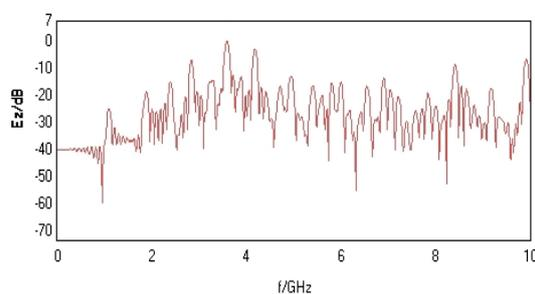
Figure 7. Electric Field in Frequency Domain of the Center of the Cavity
