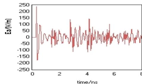
Figure 8. Electric Field of the Place 3cm to the Aperture in the Cavity when  $L=40\text{MM}$ ,  $W=6\text{mm}$
