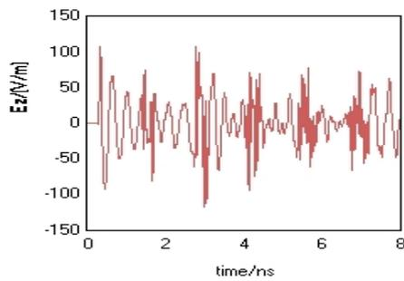
Figure 3. Electric Field of the Place 3cm to the Circular Annular Aperture in the Cavity
