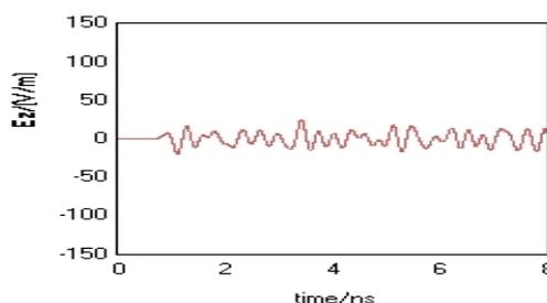
Figure 10. Electric Field of the Center of the Cavity when Pulse width is 500ps
