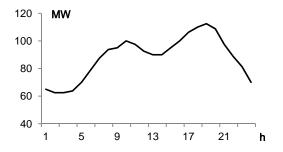
Figure 1. 24 hour daily load curve of micro-grid
