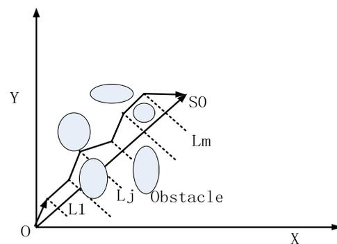
Figure 4. The Model of Path Planning
