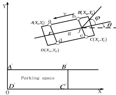
Figure 1. The Kinematic Model of the Vehicle
