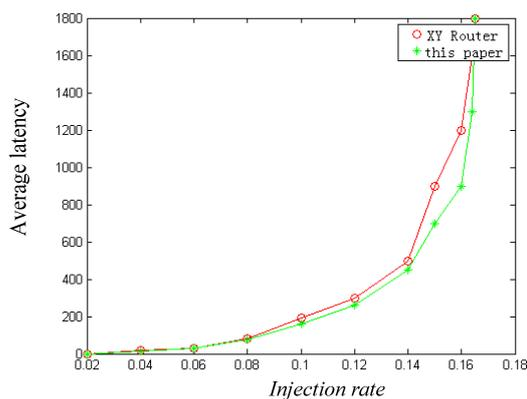
Figure 7. Average Delay of Packet Transmission
