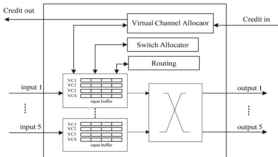
Figure 3. The Diagram of Flow Control in One Node
