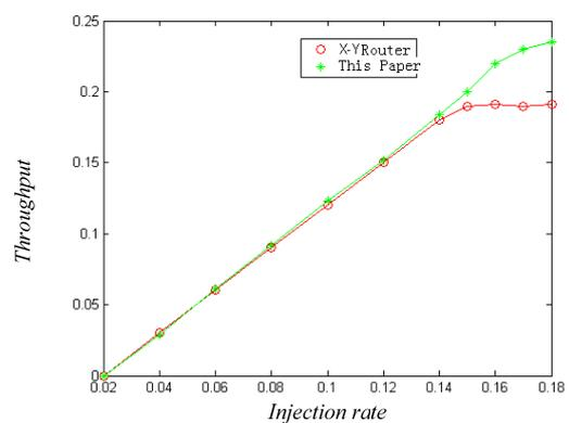
Figure 8. Throughput of Network on Chip
