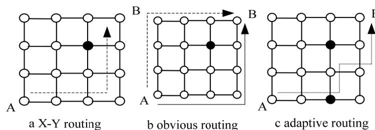
Figure 2. Network-on-chip Routing Algorithm
