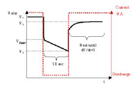
Figure 2. HPPC Test Profile
