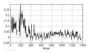
Figure 11. SOC Estimation Error Curves with EKF Algorithm
