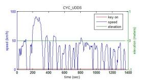
Figure 7. EPA Urban Dynamometer Driving Schedule (UDDS)
