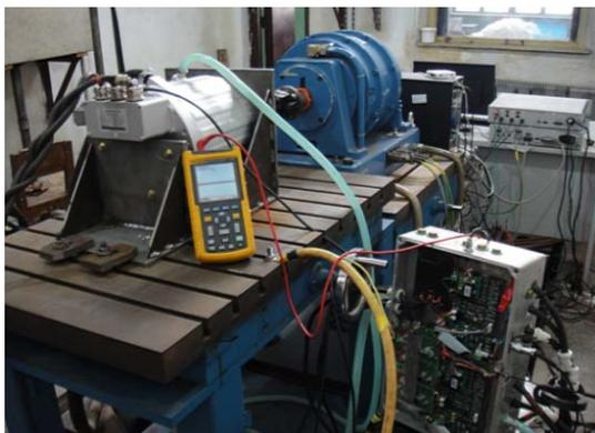
Figure 9. Picture of drive motor experiment platform
