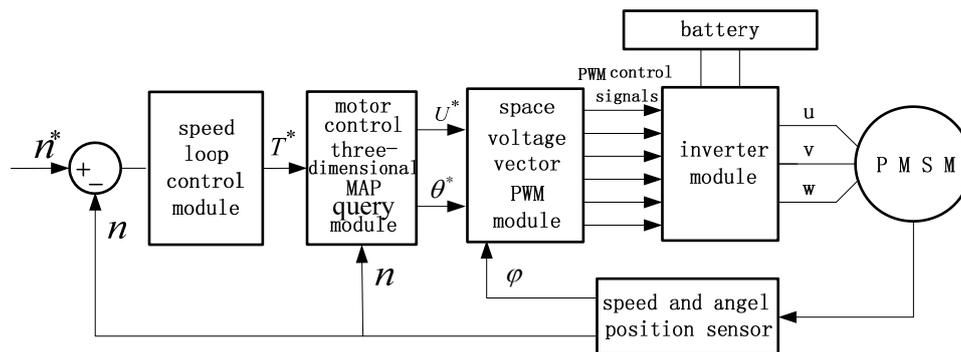
Figure 1. Schematic diagram of drive motor control system
