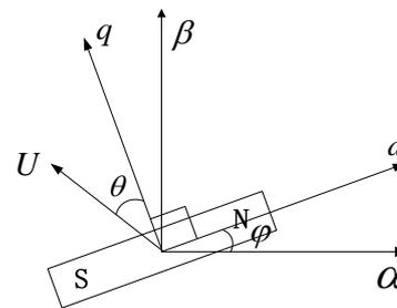
Figure 3. Vector control coordinate system
