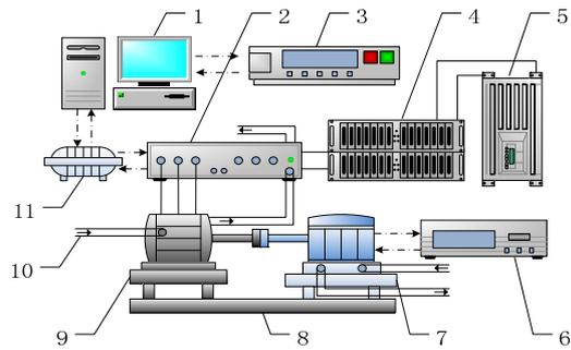
Figure 8. Drive motor experiment platform system
