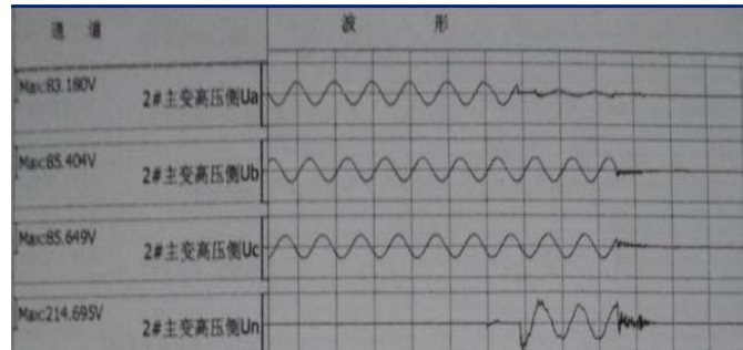
Figure 1. The Wave-recorded Information of 750kV Wusheng Substation
