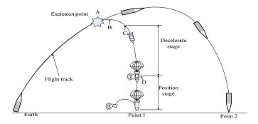
Figure 3. Schematic Diagram of the Rocket and Memory Flight Path
