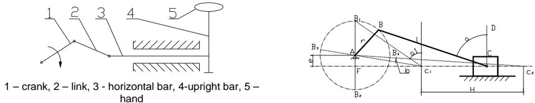
(a) structure diagram of horizontal movement (b) slider-crank mechanism analysis chart
