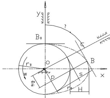
Figure 4. Analysis Chart of Flat-bottomed Putting Cam Mechanism
