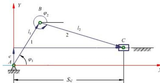
Figure 6. Analysis Chart of Slider-crank Mechanism Motion
