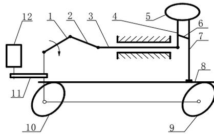
1 - crank ,2 - link ,3 - horizontal bar, 4-upright bar, 5 – hand, 6 - connecting rod, 7 - vertical bar, 8 - horizontal plate, 9 - cam1,10 - cam 2, 11 - belt, 12 –electromotor box
