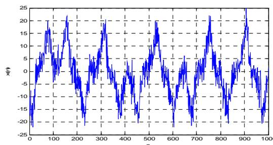
Figure 2. The Time-domain Waveform Before Noise Reduction when SNR is -10dB
