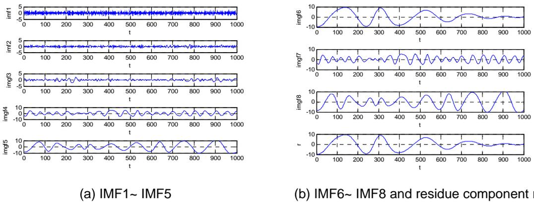
Figure 6. IMFs Derived from the Noisy Lorenz Signal by the EMD Method when SNR is 0dB
