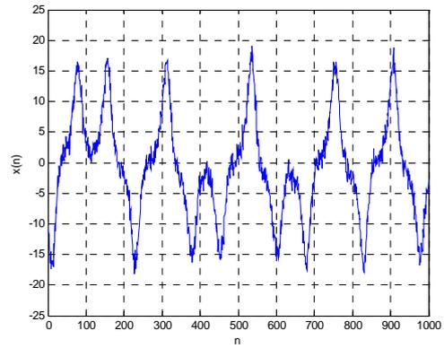
Figure 5. The Time-domain Waveform Before Noise Reduction when SNR is 0dB
