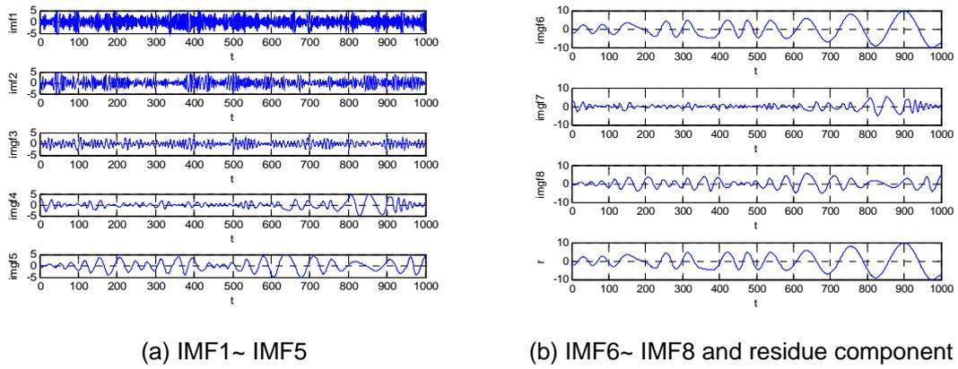
Figure 3. IMFs Derived from the Noisy Lorenz Signal by the EMD Method when SNR is -10dB
