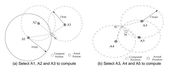
Figure 2. The Scheme of Selecting Different Beacon Nodes
