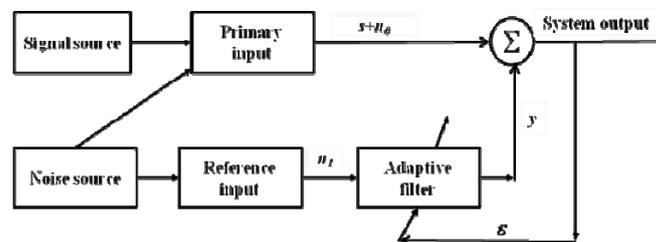
Figure 1. The Schematic Diagram of Adaptive Noise Canceller
