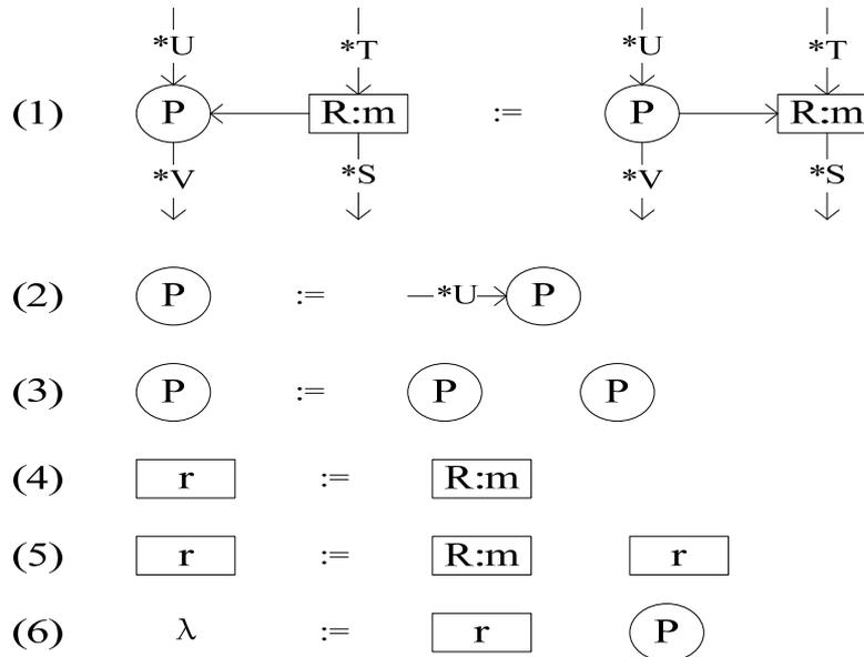
Figure 4. A set of the Rule to Construct the Test for Process Deadlock
