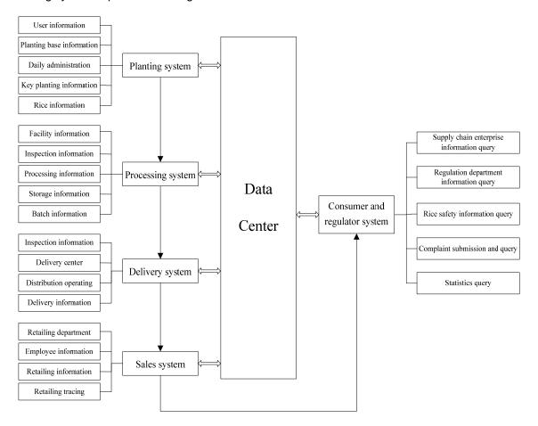
Figure 2. Information Flow of Organic RFID-based Rice Supply Chain Tracing System
