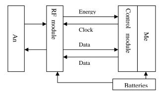
Figure 1. Structure of RFID System
