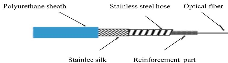
Figure 3. Structure of Armored Cable
