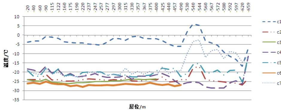
Figure 5. Curves of Thermometer Hole Temperature
