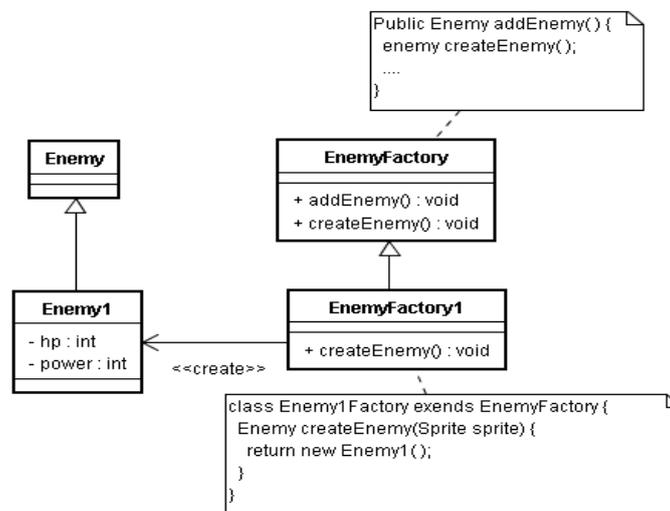
Figure 4. Factory Method Pattern
