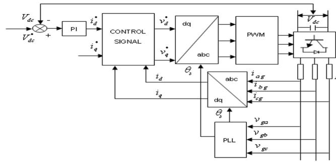
Figure 4. Vector Control Structure for GSC
