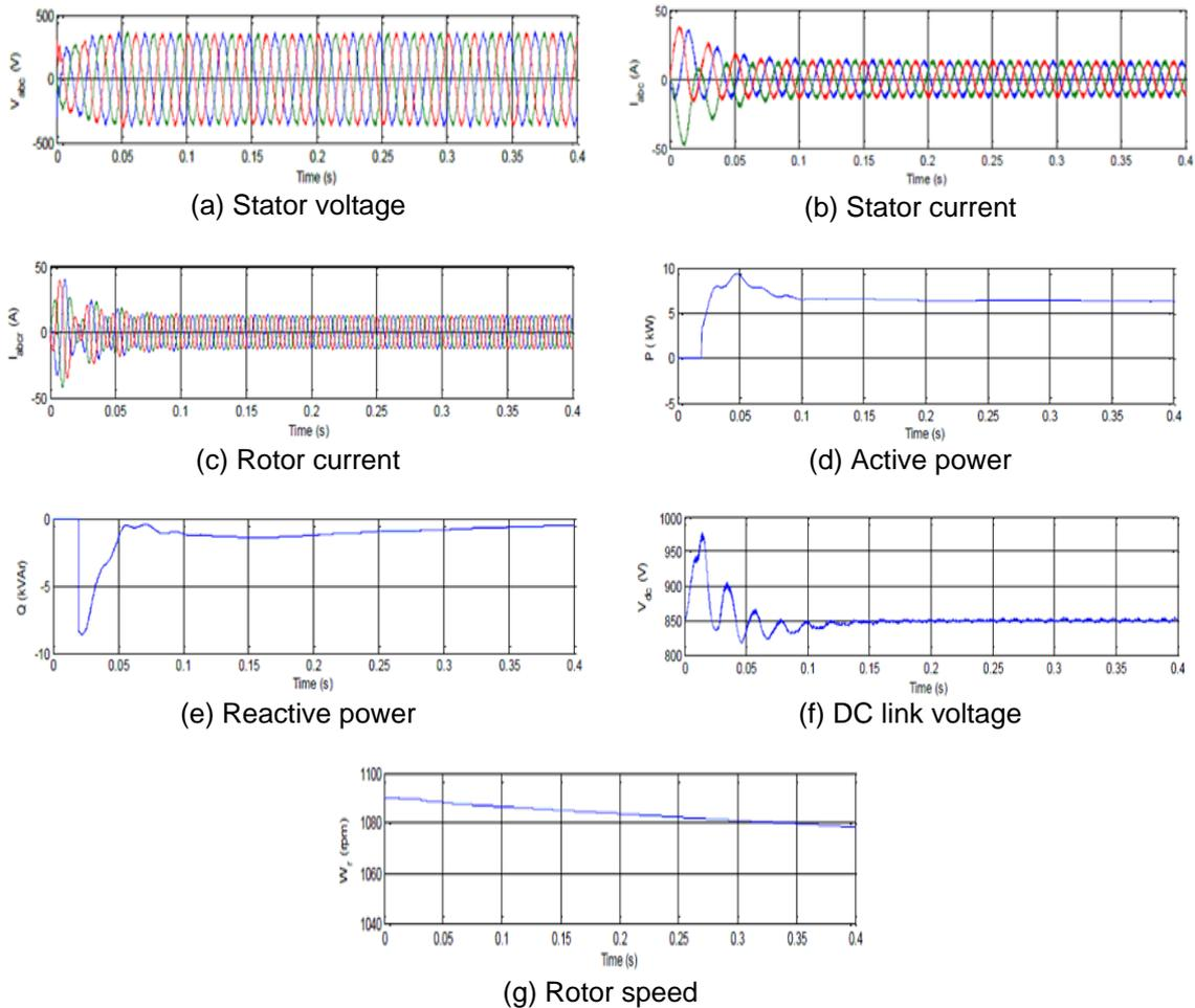
Figure 6. Simulation Results of the Grid under Balance Condition
