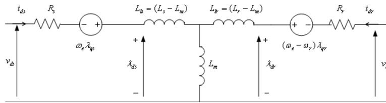
Figure 3. Dynamic d-q Equivalent Circuit of DFIG (d-axis circuit)
