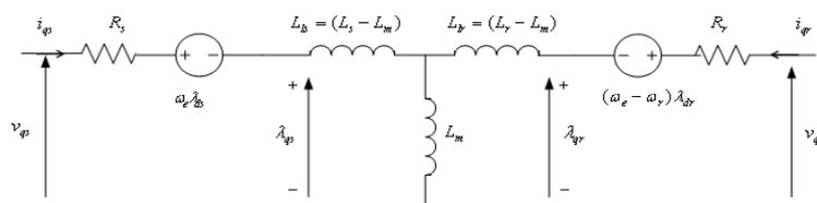
Figure 2. Dynamic d-q Equivalent Circuit of DFIG (q-axis circuit)
