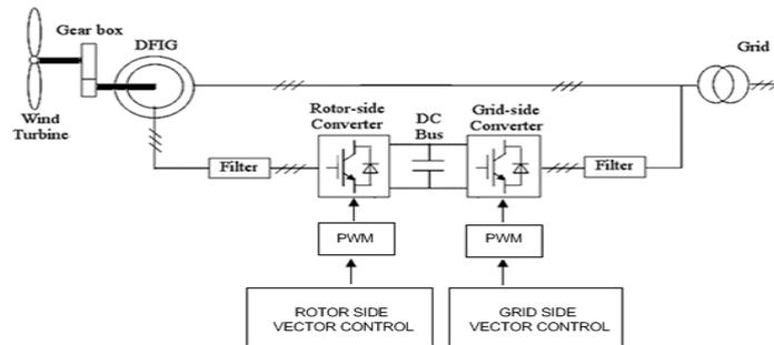
Figure 1. General Structure of Wind Power Generation System with DFIG
