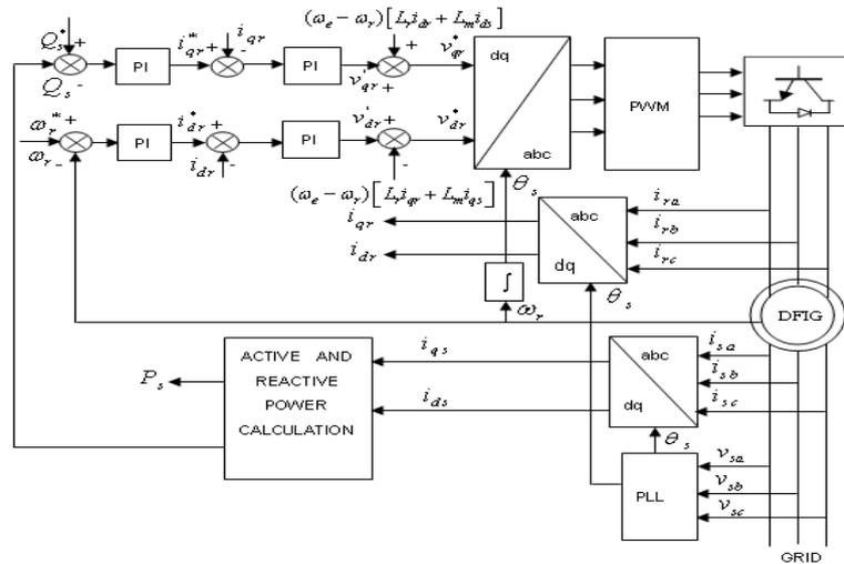
Figure 5. Vector Control Structure for RSC
