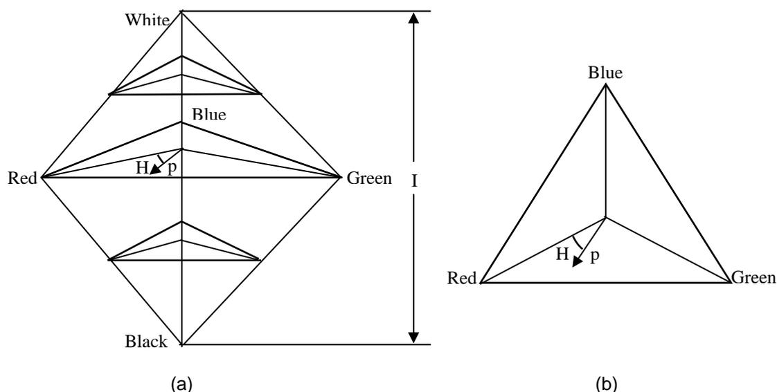
Figure 1. HSI Color Model (a) HSI 3-dimension color space, (b) cross-section of HSI color space
