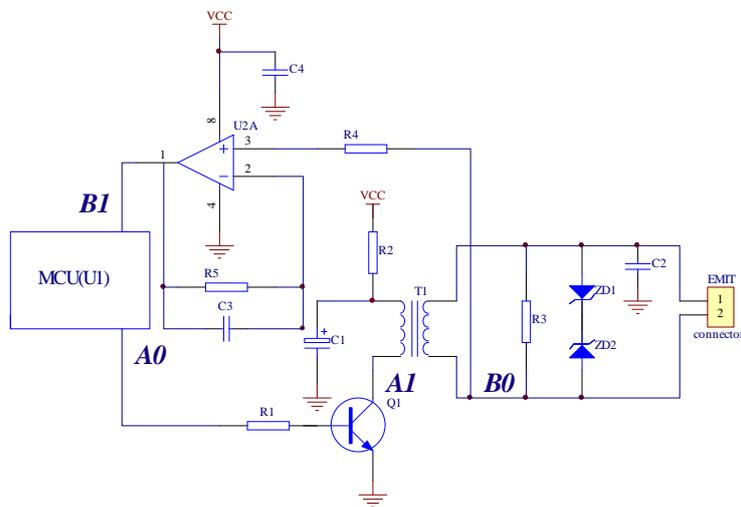
Figure 2. Sensor Signal Transceiver Schematic Diagram
