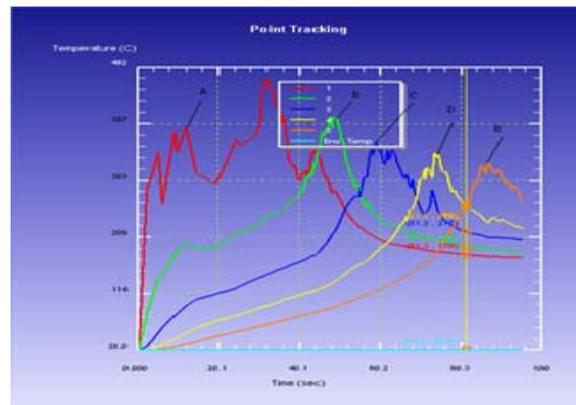
Figure 9. The Simulation Result of Temperature History of Mid Weld Point
