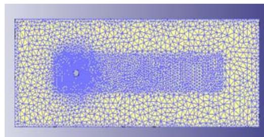
Figure 4. FEM Mesh Generation Layout Plan for Workplate
