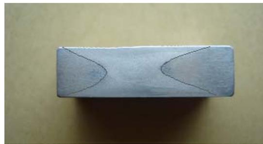
Figure 7. Macro Photo of the Weld Specimen Cross Section (X-Z) after Etching
