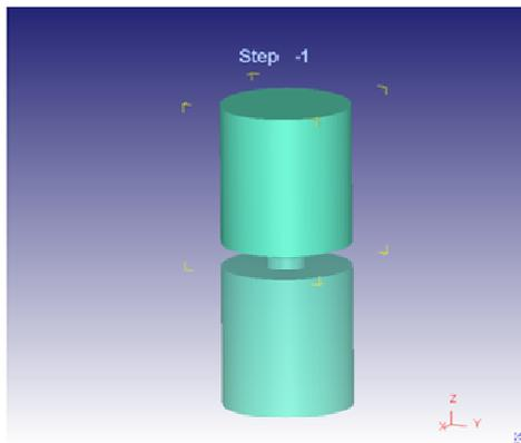
Figure 3. Bobbin Tool Geometry Model
