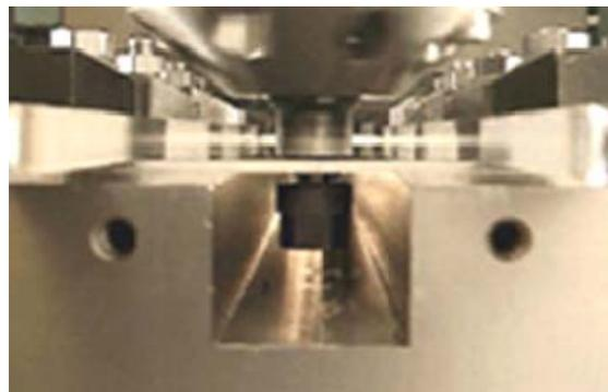
Figure 2. Photograph of Bobbin Tool Friction Stir Welding [7]
