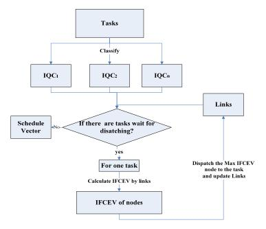
Figure 2. The Flow Chart of the IFS-QoS PA Algorithm
