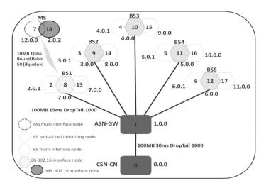
Figure 5. Horizontal Handover with Node ID and IP Addressing
