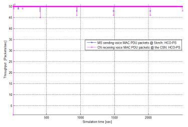
Figure 8. Throughput for Pedestrian Speed at Half-cell Overlap Coverage
