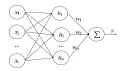
Figure 1. RBF Neural Network Prediction Model Structure
