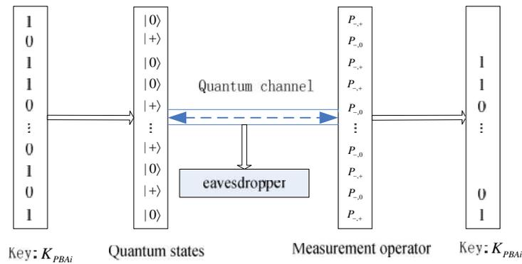
Figure 3. Periodic Communication Quantum Channel Based on the Improved B92
