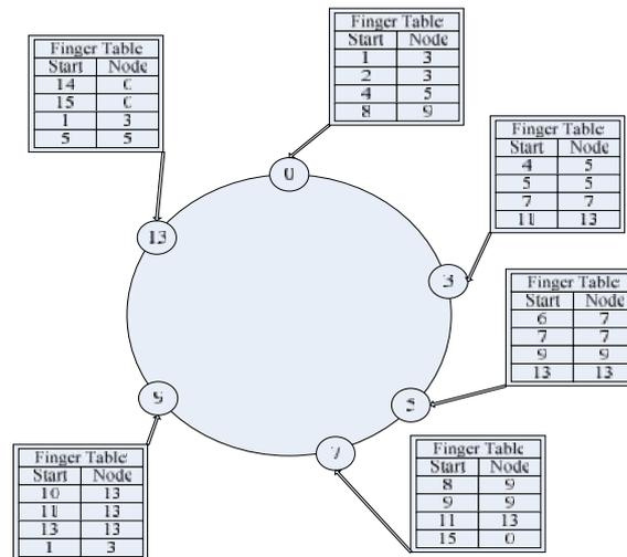
Figure 1. Network Topology of Chord-based Botnet
