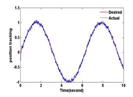
Figure 6. Position trajectory without filter
