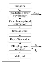
Figure 5. The flow chart of kalman filtering
