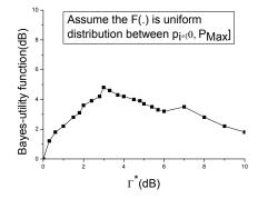
Figure 2. The optimal SINR threshold  $p_i \in [0, P_{max}]$
