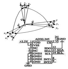
Figure 3. ADXL345 Digital Three Axis Accelerometer Structure Diagram
