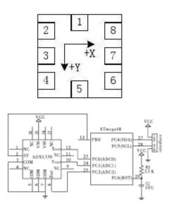
Figure 1. The Circuit Principle Diagram of Sensor Network Node
