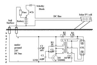
Figure 3. Fly-back inverter operating using BJT
