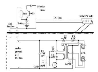
Figure 2. Fly-back inverter for operating CFL using MOSFET
