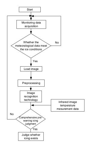
Figure 4. The comprehensive early warning method for transmission line icing
