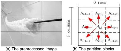
Figure 2. Diagram of space-based image segmentation
