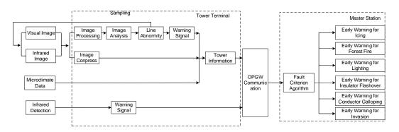
Figure 1. Online early warning system for the transmission lines
