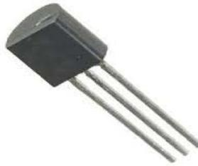
Figure 2. LM 35 temperature sensor
