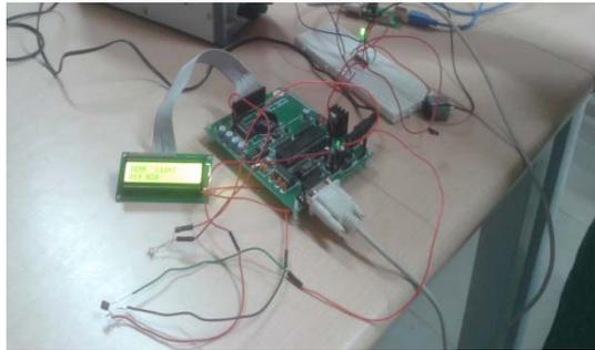
Figure 4. interfacing of sensors with the micro controller
